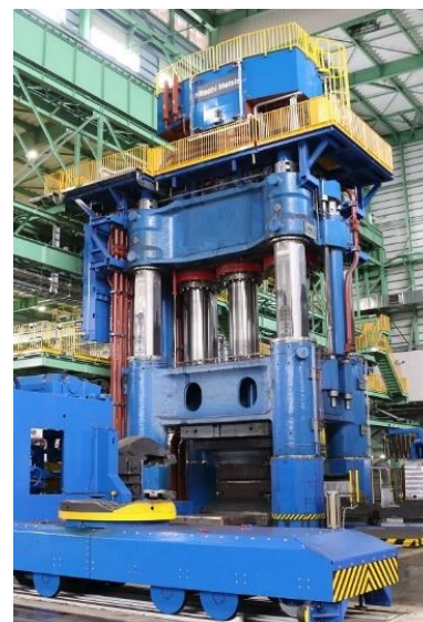
10,000-ton free forging press
